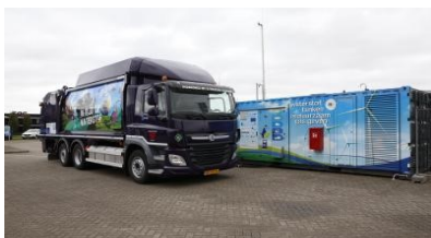
1. Mobiel H 2 -tankstation 2
