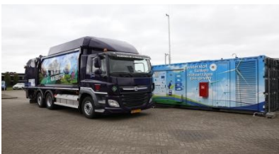
1. Mobiel H 2 -tankstation 1
